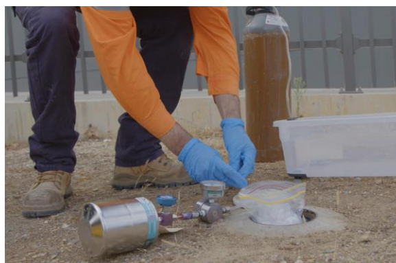
Sampling a soil vapour bore
