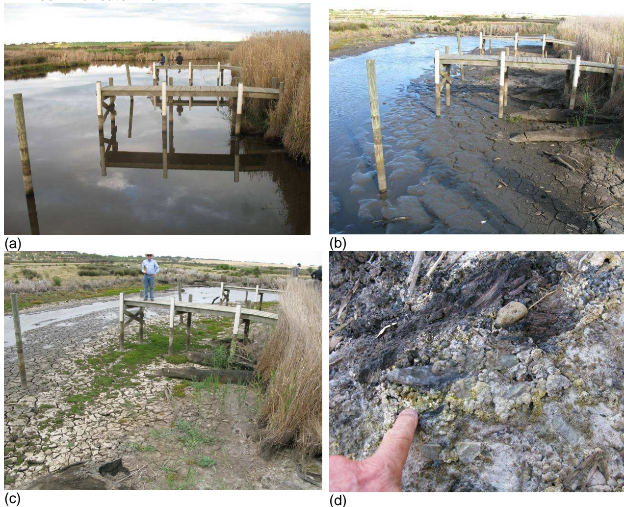
Figure 5. Changes in water level in the Finniss River at Watsons Landing, which is the sampling site furthest upstream on the western side of the Finniss River (labelled as FIN 26 in Figure 1). a) August, 2007 showing the whole river ponded with water. A sulfidic subaqueous clayey soil was sampled under 80 cm of water at the end of the jetty and labelled as sample AA 26; Sulfidic organic clayey soil was sampled in the Phragmites four metres from the bank/waters edge and labelled as sample AA27 (see Fitzpatrick et al. 2008b pp. 99 and 118 for morphological and chemical data respectively). b) November 2008 showing substantial lowering of water levels to produce mainly waterlogged or saturated ASS (sulfidic cracking clay soil – end of jetty). c) January 8 th 2009 showing further lowering of water levels to expose a clayey dry river-bed with cracks and salt efflorescences (sulfuric cracking clay soil). d) November 2008 showing close-up photograph of the dry clayey river-bed adjacent to the Phragmites in the river bank. White fluffy salt efflorescences (comprising mixtures of mainly Mg-sulfate minerals [hexahydrate \text{MgSO}_4 \cdot 6\text{H}_2\text{O} , epsomite \text{MgSO}_4 \cdot 7\text{H}_2\text{O} ] and gypsum) and bright yellowish green coloured iron oxyhydroxysulfate minerals comprising sideronatrite [\text{Na}_2\text{Fe}(\text{SO}_4)_2 \cdot \text{OH} \cdot \text{H}_2\text{O}] , tamarugite [\text{NaAl}(\text{SO}_4)_2 \cdot 6\text{H}_2\text{O}] with pH values of 1.6 to 2.5 overlying clayey sulfuric material (sulfuric cracking clay soil) (see Appendix 1 for XRD).
