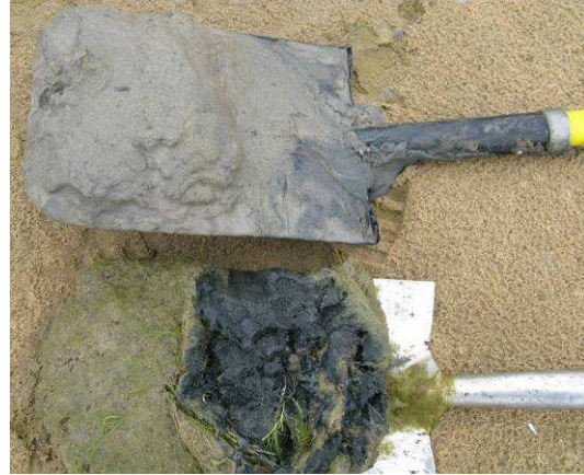
Figure 13. Sandy sulfidic subaqueous soil in Currency Creek showing black monosulfidic black ooze (MBO) beneath green algal mat. (Site CUR 22 on Figure 1).
