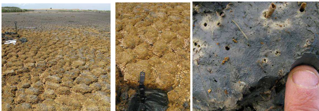
Figure 8. Acid sulfate soil in the clayey dry river-bed of the Finniss River (Site FIN 28 on Figure 1) showing a soil pit with black sulfidic material (iron sulfides) at depth (> 60 cm) overlying sulfuric material with pale yellow mottles surrounding old Phragmites root channels in a dark grey matrix consisting of jarosite (right hand side) overlying a cracked surface layer comprising mainly the bright orange mineral, schwertmannite (Appendix 1), which has a pH ranging between 3 and 3.6.
