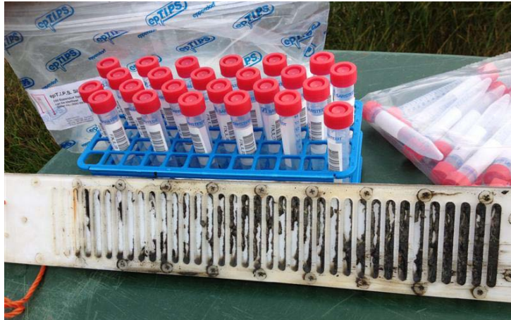
Figure 3 A peeper following retrieval, ready to be rinsed and the filling solution in the chambers extracted
