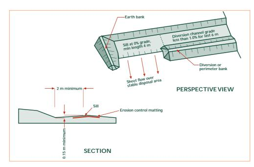
Figure 5.3 Level spreader installation method.
