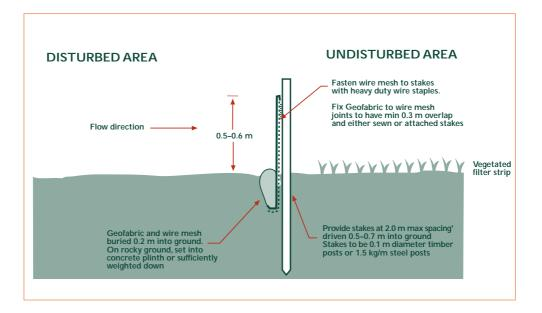
Figure 5.5 Silt fence installation method.
