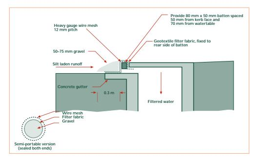
Figure 5.7 Side inlet pit trap.
