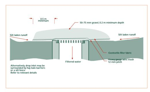
Figure 5.6 Drop inlet pit trap.
