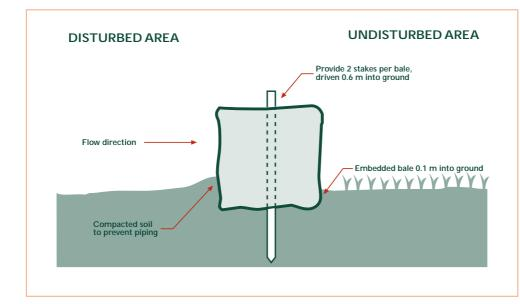
Figure 5.4 Hay bale installation method.
