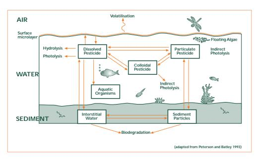
Figure 3.1 Pesticide transport and transformation processes.
