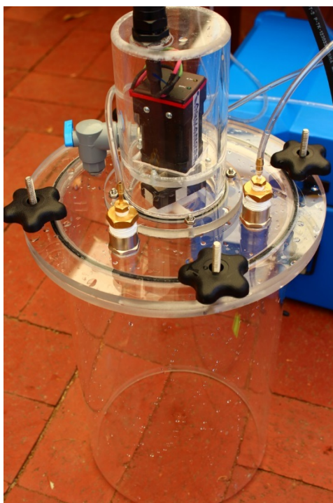
Figure 2 A photo taken prior to field testing of chamber one. The equipment included the head unit (electronic components), magnetic stirrer, gold taps, airline tubing, tie down points for weights and the series of o-rings and flanges separating each component are visible. Note there is no white collar present on this chamber.
