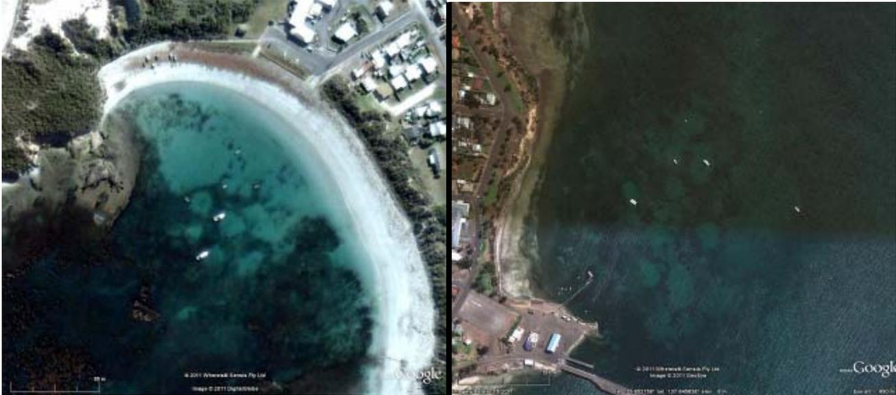
**Figure 1** Circular scours in seagrass meadows in the South East and Kangaroo Island of South Australia. Circular scours particularly in close proximity to boat anchorages have been shown to be symptomatic of loss due to scour caused by swing boat moorings (Walker et al 1989; Hastings et al 1995) .
