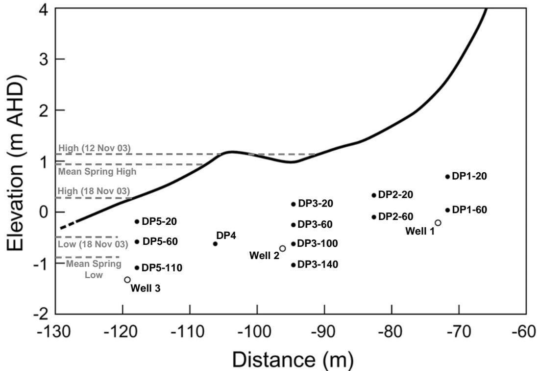
**Fig. 2.2.** Cross-section of the West Beach beachface transect sampled on 18 November 2003. Open circles are for the wells and closed circles represent drive points (with the number following the drive points the approximate distance from the water table in cm). Distances are in metres along a SW – NE transect perpendicular to the shoreline, with the SA Department of Lands Survey Mark 6528 2036 as the origin. Also indicated are representative tide heights (Port Adelaide Outer Harbour).
