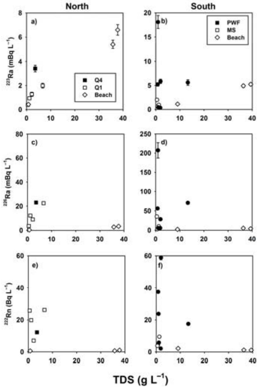
**Fig. 3.2.** Activities of <sup>223</sup>Ra, <sup>226</sup>Ra and <sup>222</sup>Rn in regional groundwater and beachface groundwater as a function of salinity.
