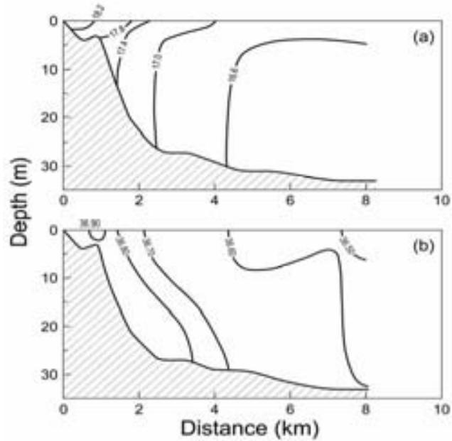
**Fig. 3.4.** a) Temperature (°C) and b) salinity profiles (as TDS, g L<sup>-1</sup>) at the Northern Transect, 4 November 2003.
