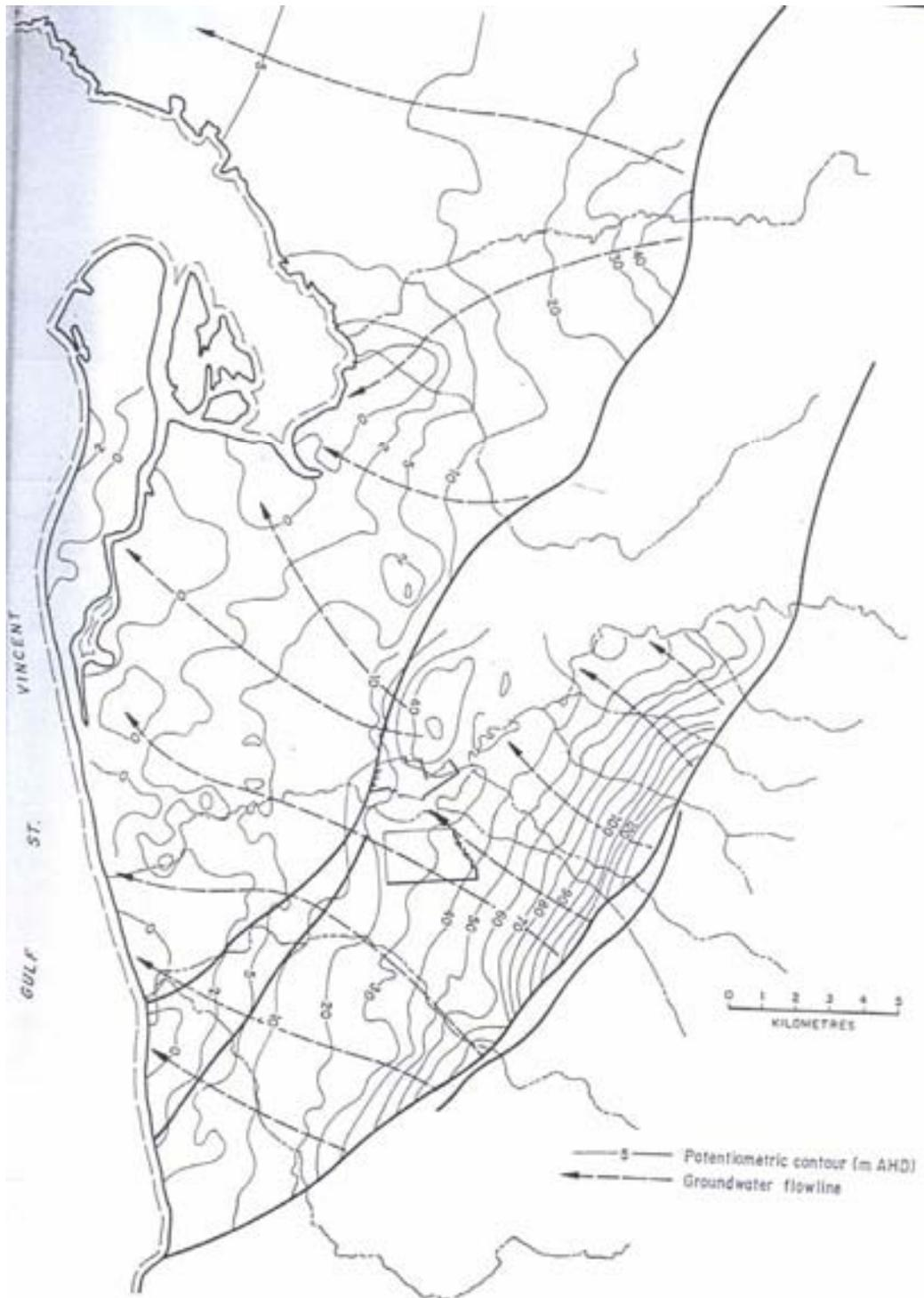
**Fig. 1.10.** Generalised potentiometric surfaces for the shallow Quaternary system in Metropolitan Adelaide (Pavelic *et al.* 1992).
