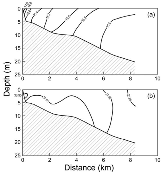
**Fig. 3.5.** a) Temperature (°C) and b) salinity profiles (as TDS, g L<sup>-1</sup>) at the Southern Transect, 26 November 2003.
