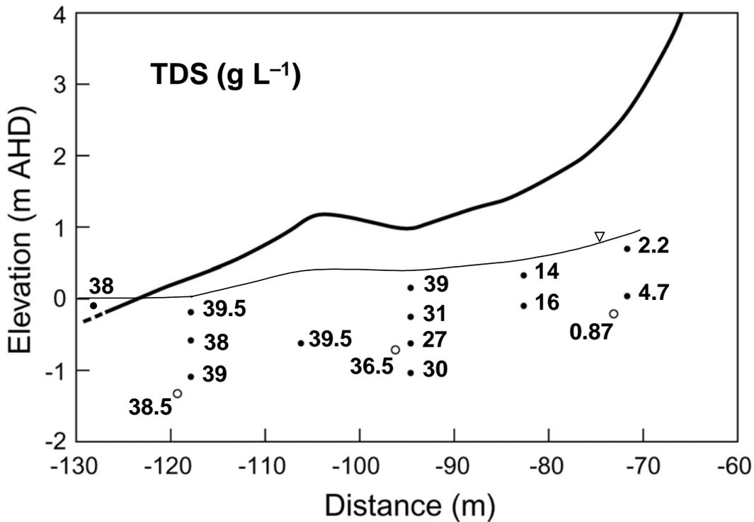
**Fig. 2.3.** Salinity (as TDS) along the West Beach beachface cross-section. The inverted triangle shows the position of the water table.
