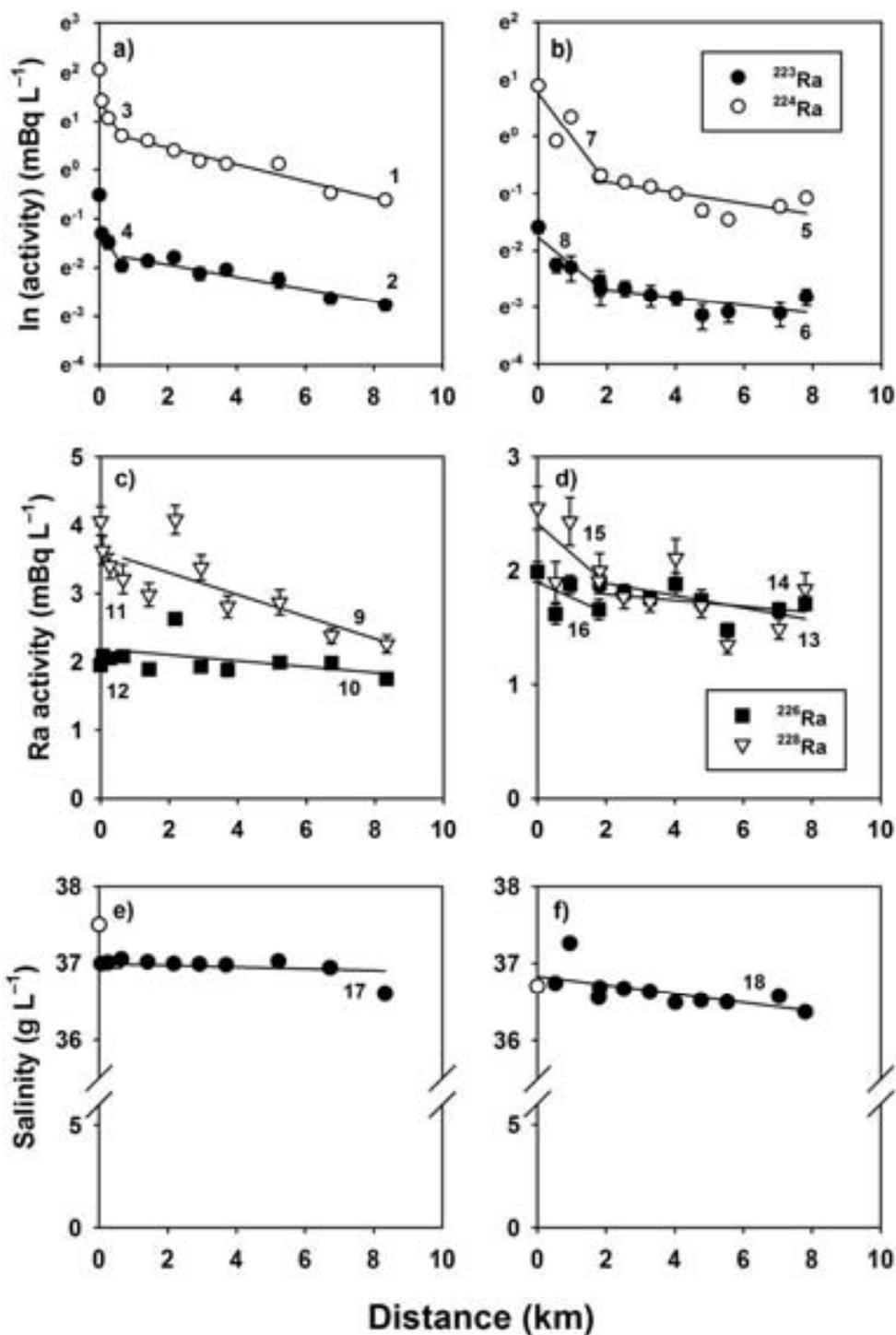
**Fig. 3.8.** Estimation of the gradients in Ra activity and in salinity with distance offshore. Short-lived Ra isotopes for the a) Northern and b) Southern transect, long-lived Ra isotopes for the c) Northern and d) Southern transect and surface salinity for the e) Northern and f) Southern transect. See Table 3.4 for the summary of the regression statistics. Open circles on e) and f) represent data collected with a less accurate hand held meter.
