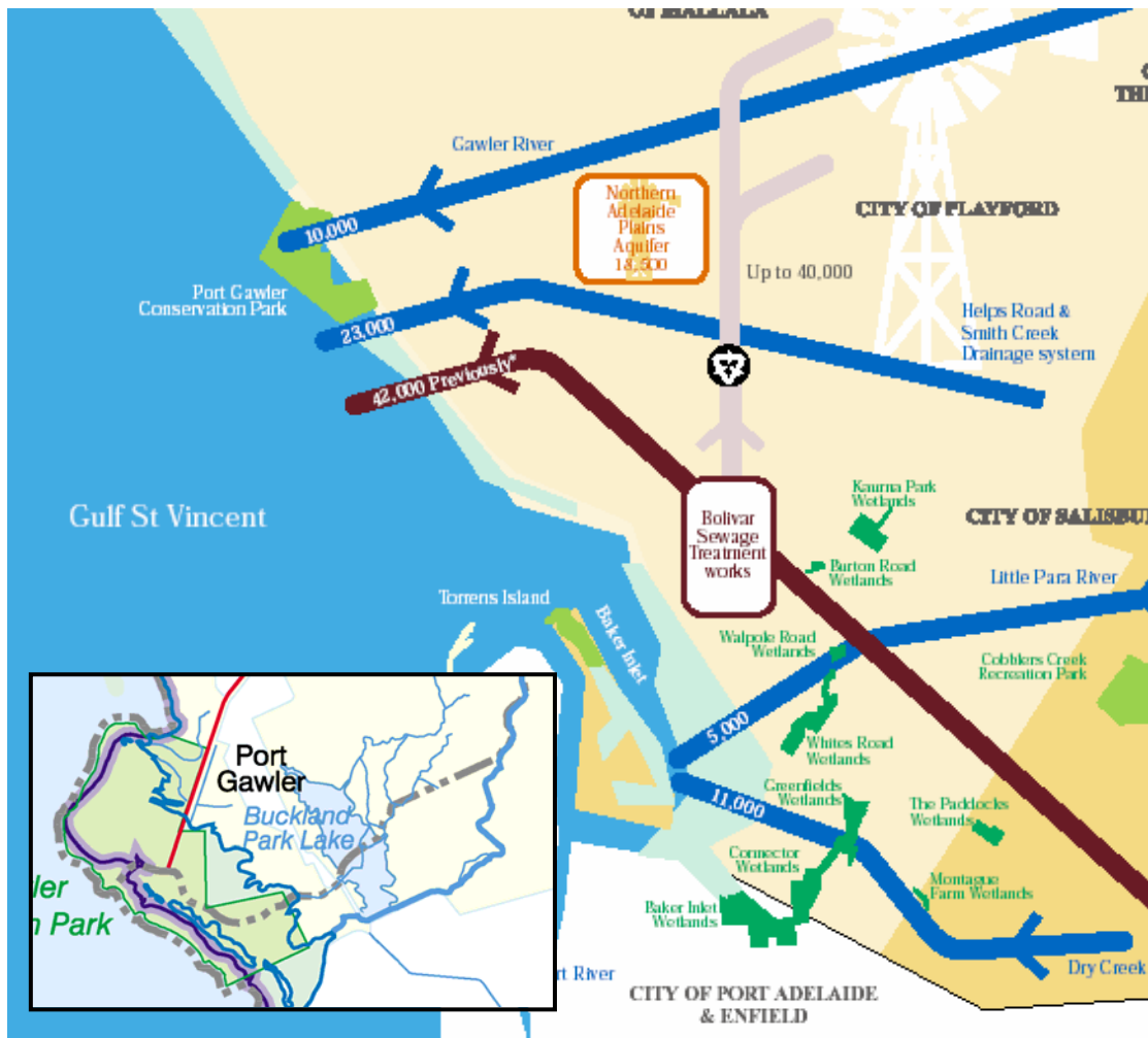
Figure All.3 Section of water balance schematic for the Gawler River and Smith Creek (From the NABCWMB Plan 2001-6). The inset shows Buckland Park Lake.
