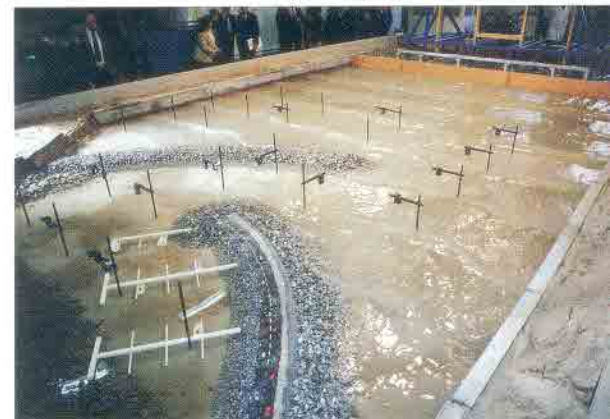
Wave modelling tank used to test marina design
