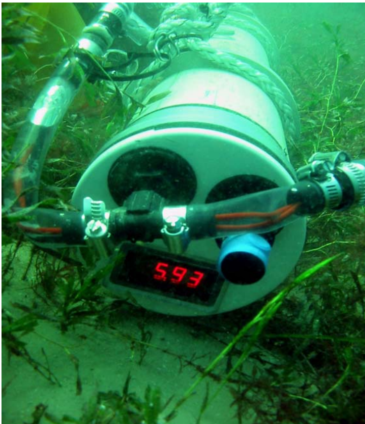
Close-up of the high amperage underwater battery pack
