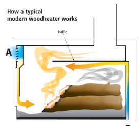
Primary air [A] is drawn in through a sliding or hinged air control mechanism, usually above the door. The air is preheated before being directed down the inside of the door, helping to keep the glass clean. It then enters the base of the fire. This primary air supply determines how quickly the firewood burns.
