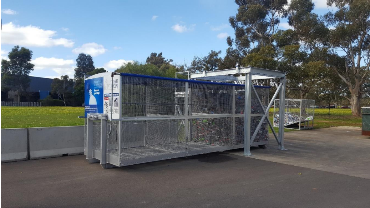
Figure 6: Example photo of roll-on/roll-off CDS container cage from a MRF that would be transported directly to a Super Collector facility for baling and sending to markets for recycling
