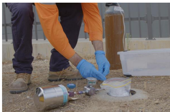
Sampling a soil vapour bore
