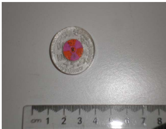
Figure 1 Image of a typical sealed source found in schools, known as a 'button source'. They are usually made from either americium (alpha emitter), strontium (beta emitter) or cobalt (gamma emitter).
