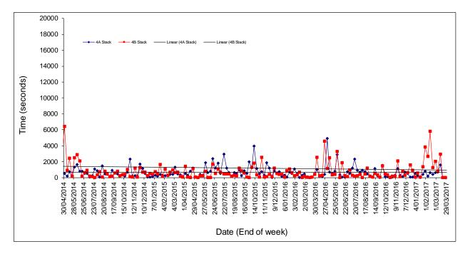
Tracking total time for stack emissions greater than the reporting levels of 150mg/Nm<sup>3</sup> on 4A stack and 80mg/Nm<sup>3</sup> on 4B stack.
