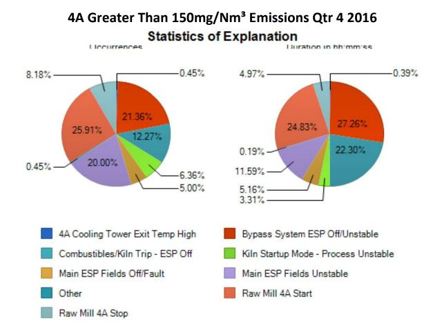
4A Stack Pie Chart of causes over 150 mg/Nm<sup>3</sup> in terms of number of occurrences and total time
