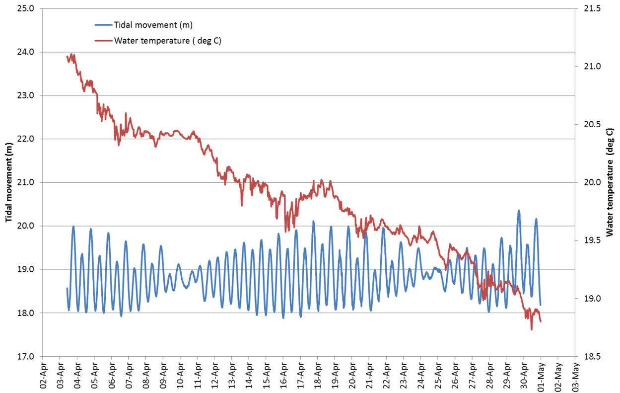
**Figure 5.** Changes in dissolved temperature (°C) with tidal movement (m) over 28 days, from 3<sup>rd</sup> April to 30<sup>th</sup> April 2014.
