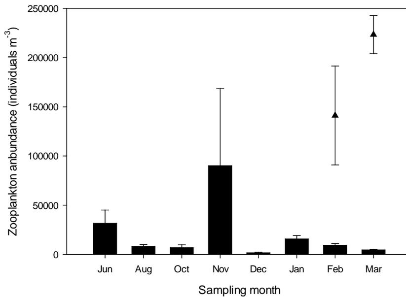
Figure 6. Mean zooplankton abundance in samples collected from the intake tunnel of the Adelaide Desalination Plant (ADP) prior to the band screens (bars), and offshore at the intake riser pipe (triangles) in 2013/2014. Error bars indicate standard error.
